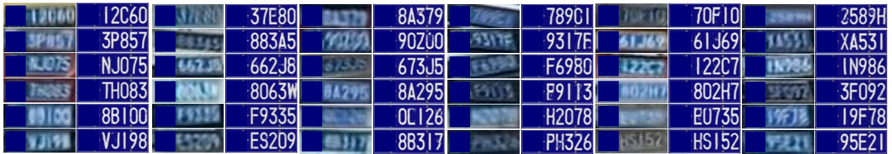
Figure 2: Some results of the proposed multiple license plates super-resolution with progressive vehicle search and domain priori GAN. Even for the plate images which cannot be recognized by humans, our method can well recover their high-resolution images.
