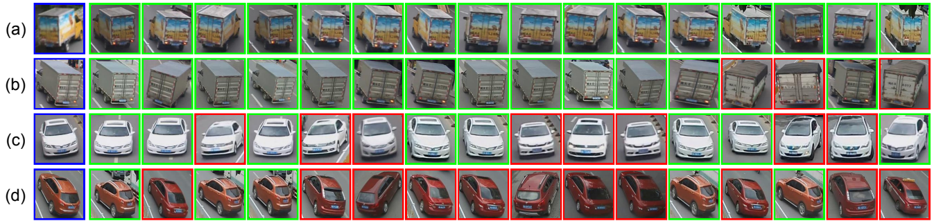
Fig. 5. Sample results of the FACT on VeRi dataset. The query is in blue box and the top-16 results are listed. The true positive results are in green box, otherwise red.
